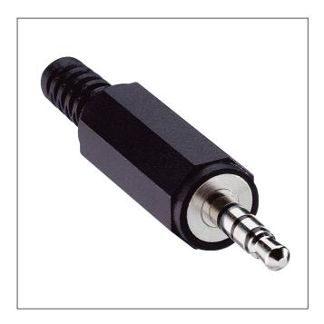
Jack plug according to JEITA RC-5325A JC35P4, 3.5 mm, 4 poles/stereo, straight version, with bend protection and solder terminals
